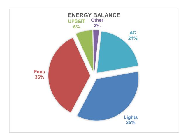
36 % of the total energy consumed in this facility is used to operate Fans. Lighting uses 35% AC uses 21%, Others uses 13% and IT Equipment uses 4%.
